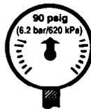
**Operate at 90 p.s.i.g. (6.2 bar/620 kPa) maximum air pressure.**
