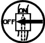
**Turn off air supply and disconnect air supply hose before installing, removing or adjusting any accessory on this tool, or before performing any maintenance on this tool.**
