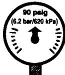
Operate at 90 p.s.i.g. (6.2 bar/620 kPa) maximum air pressure.
